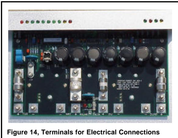
Figure 14, Terminals for Electrical Connections
