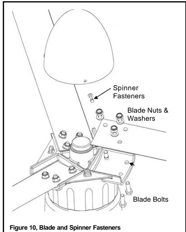
Figure 10, Blade and Spinner Fasteners
