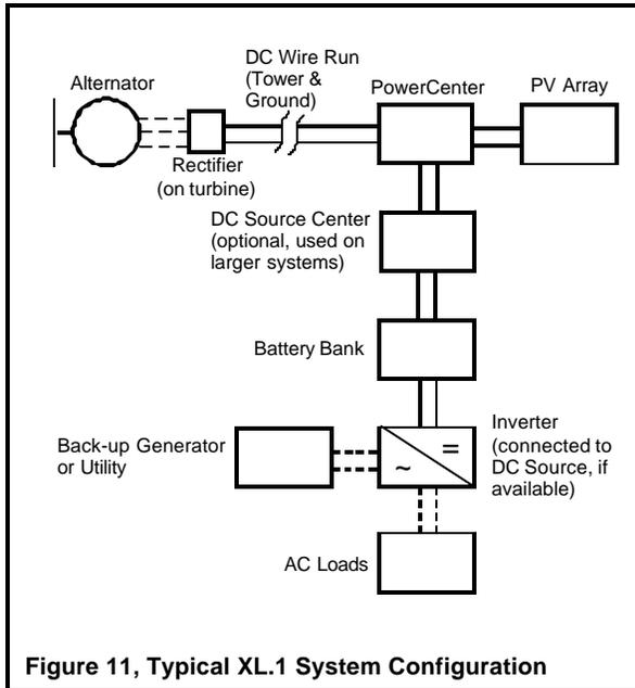
Figure 11, Typical XL.1 System Configuration
