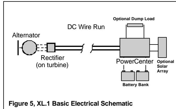
**Figure 5, XL.1 Basic Electrical Schematic**
