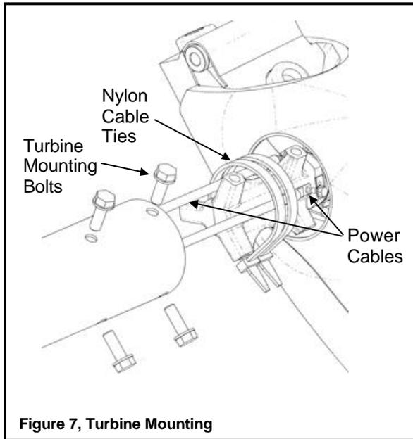
Figure 7, Turbine Mounting
