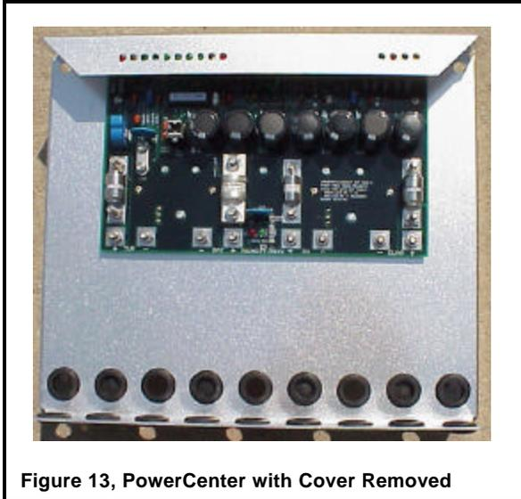
Figure 13, PowerCenter with Cover Removed
