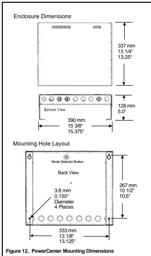
Figure 12, PowerCenter Mounting Dimensions
